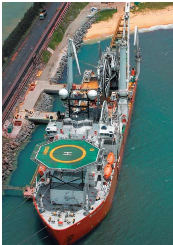
Seven Oceans during spooling operations at Ubu Spoolbase, Brazil
