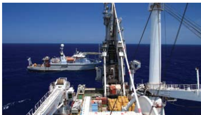
Seven Oceans Laying pipe and Seisranger performing touch-down monitoring
